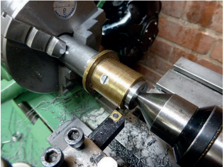
Machining the OD of the top bush
