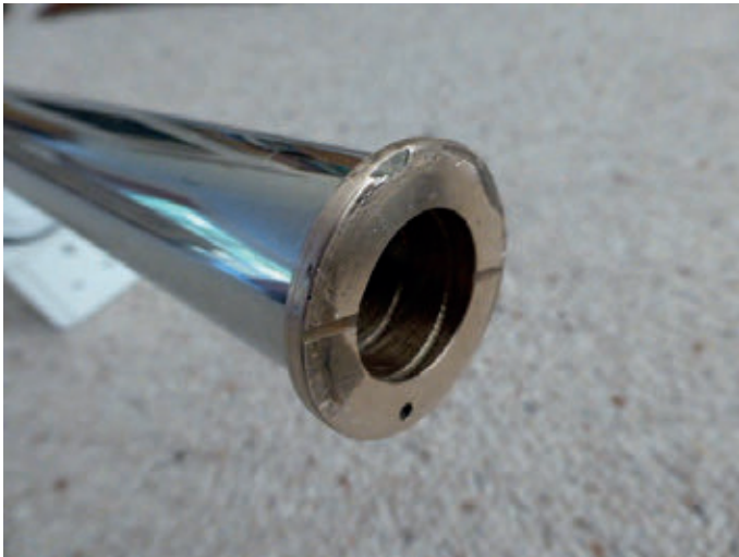
Top bush installed
